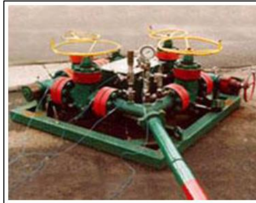
Figura 7: Choke manifold.
